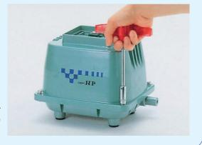
Replacing the Chamber Block
